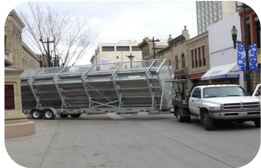
Folding & Mobile State Can be transported by truck in highway
